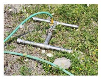
Figure 4 Coarse Bubble Aerator
