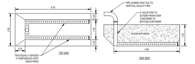
Figure 6 Biofilter Schematic
